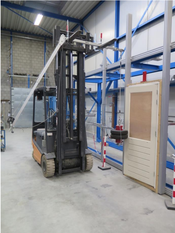
Functionality test: Impact on position of the lock
