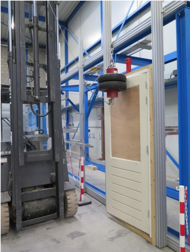
Strength and overload test: Impact on position of the stopper
